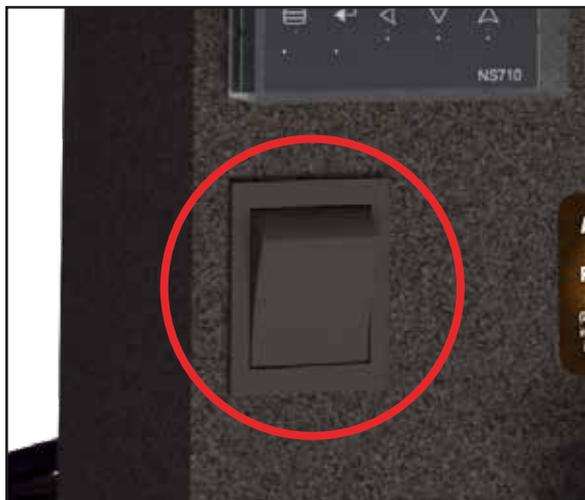
Set power switch to the “on” position. You will notice on your control screen there are two rows of digits. The top is the current temperature of the heat plates. The bottom is the set temperature. The mini comes preset at 200 degrees Fahrenheit and will take approximately 5-7 minutes to reach set temperature depending on your location.
