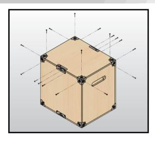
Remove the 18 screws from top fasteners of the crate.
