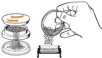
Fill the Filling Chamber to the bottom edge of the hopper at most
