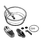
Place all parts of the Cooling Unit in warm rinsing water.
