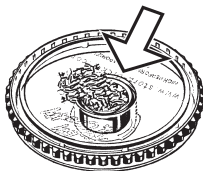
Dosing Capsule while being filled with Magazine Cap (funnel)
