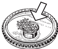
Dosing Capsule while being filled with Magazine Cap (funnel)
