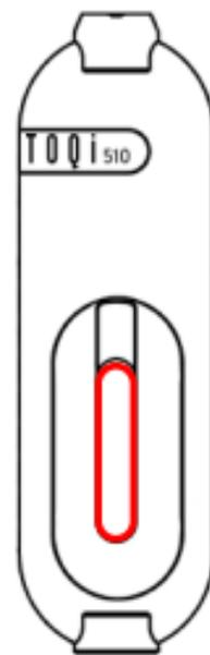
**press button two (2) times to check battery**
